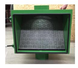
Model 2424 Filter is designed with a removable 24"x 24" screen assembly which can accommodate a variety of screens types. Inline Safety Filters are typically shipped with a 30 mesh stainless steel wire cloth which allows most dust particles to pass through while capturing the fibers that normally accumulate on the leading edges of the impellers of High Vacuum exhausters.
